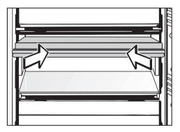
Slide the isolation plate in underneath the third drawer.
